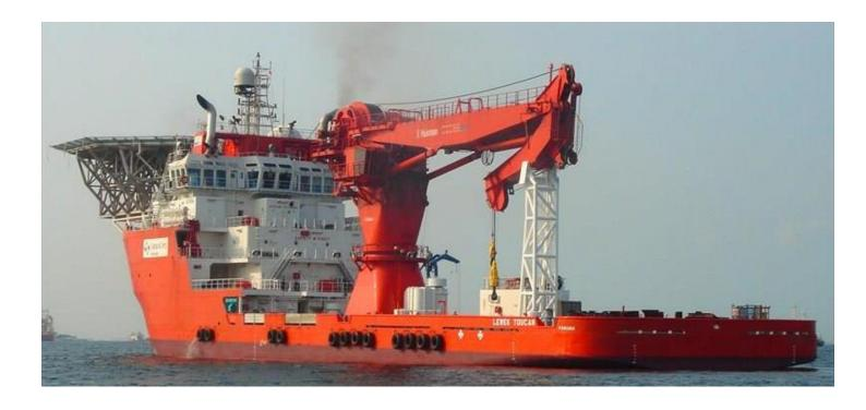
Prince Jameson I is an advanced multipurpose offshore support vessel with excellent dive support capabilities as well as a DP 2 dynamic positioning system, accommodations for a crew of 100, a 920 M2 /1,000 ton cargo deck and helideck. The 120 ton capacity crane has a 12 metres reach and is capable of operating in water depths reaching 2,000 m.
